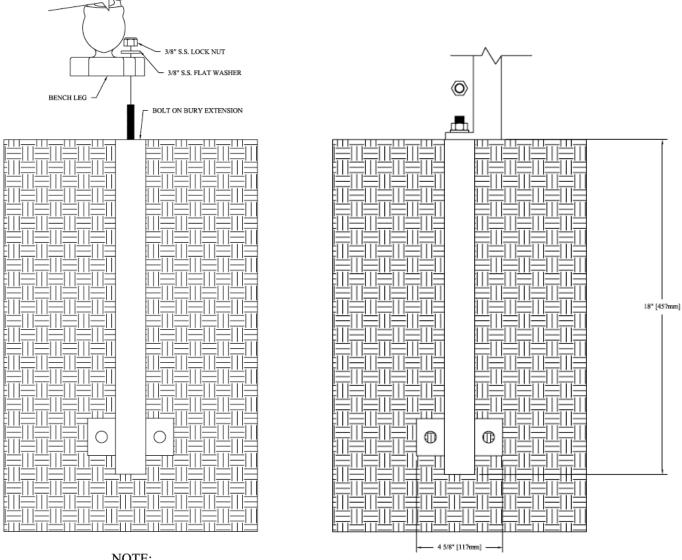
NOTE: THIS TYPICAL BURY EXTENSION CAN BE USED ON ANY ITEM WITH A CAST LEG.
